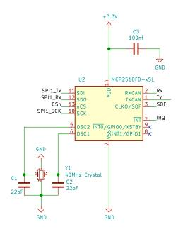
The CAN controller is clocked by a 40MHz crystal and the SPI clock from the RP2040 on the Pico can go up to 18.5MHz. More details on the SPI interface can be found in section 4 of the CAN controller datasheet (available from Microchip).
