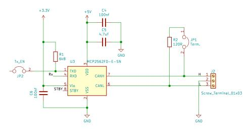
The TXD input to the transceiver comes from either the CAN controller or a GPIO pin from the Pico (the latter is to allow software to emulate aspects of the CAN protocol). The signal goes through jumper JP2 ("Tx\_EN"): if this is not closed then a pull-up resistor holds TXD high and no software can send signals on the CAN bus (this is useful if software on the Pico is to monitor a CAN bus without the possibility of disturbing it).
