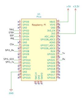
The Pico should be soldered to the CANPico at the 13 pins shown in the schematic above. The Pico has castellated ("half moon") edges to support this, allowing headers to be soldered into the holes if an additional Pico-compatible board is to be connected. The Pico SPI1 interface<sup>2</sup> is used to connect to the CANPico, leaving SPI0 free to connect to other boards.
